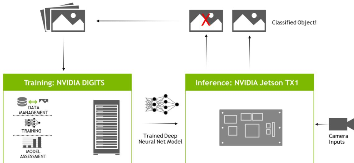
Figure 1 - Jetson-Inference block diagram
